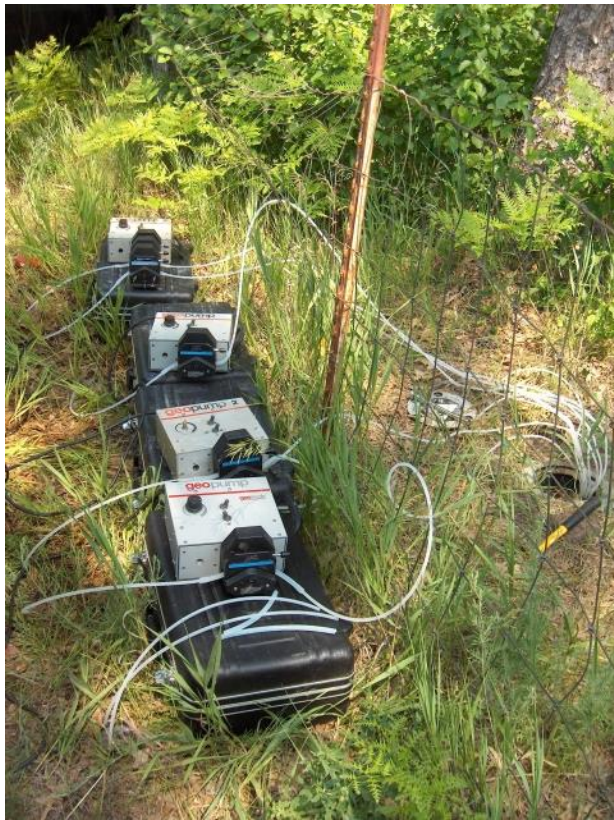
Sample with multiple pumps
